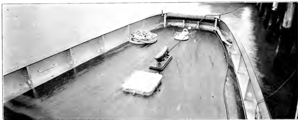
Below, after deck of the Mamo from the top of deck house; the hawser roller is equipped with Timken roller bearings.
